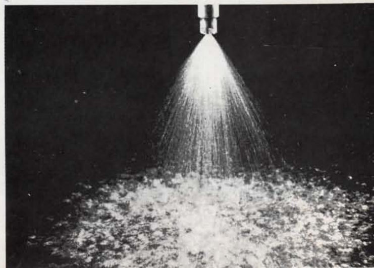
FIG. 3 — View showing square spray pattern obtained with special nozzles.
